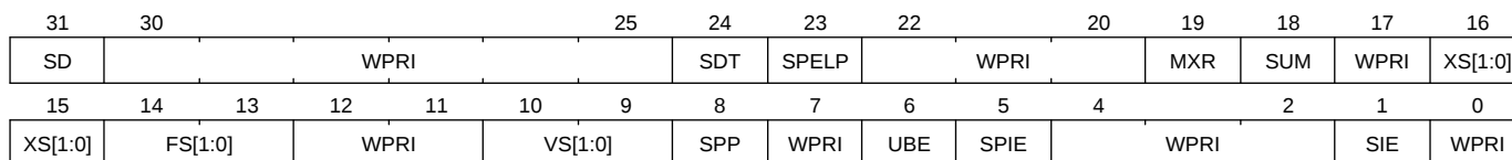
Figure 20. Virtual supervisor status ( vsstatus ) register when VSXLEN=32.
