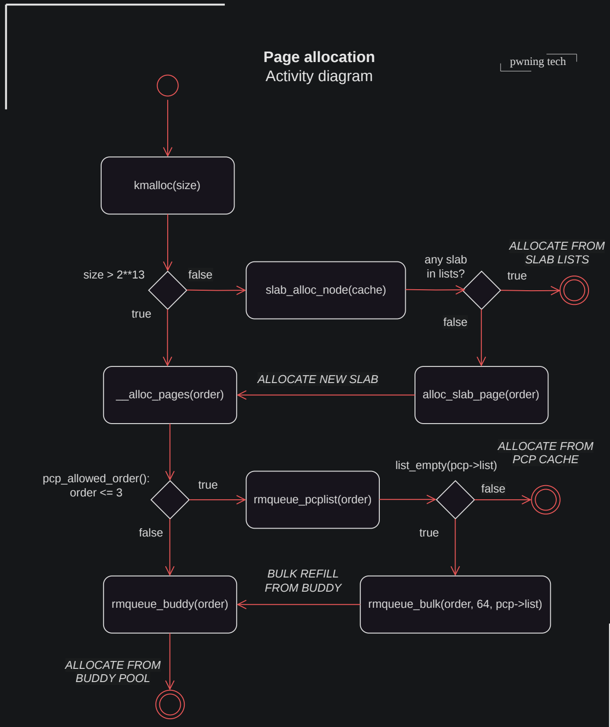
Illustration 2.4.2: Activity diagram of the page allocation process, starting from kmalloc() .
