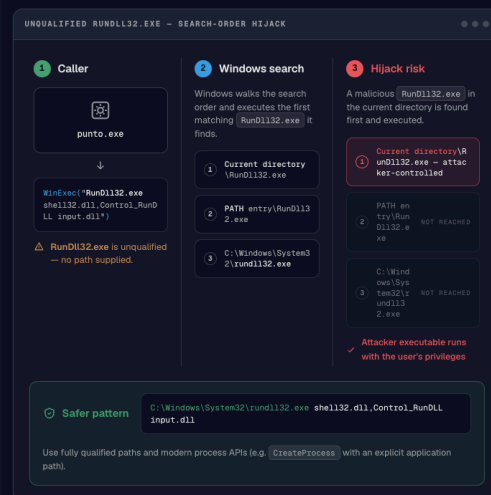
Figure 1: How an unqualified RunDll32.exe call lets an attacker-placed executable run in place of the legitimate system binary.
